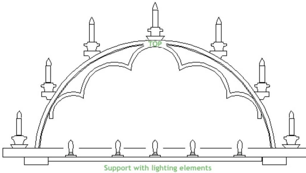
2. **Disconnect mains.** Unscrew support and **cautiously** pull out, moving it downward. Lower part of support remains between feet.
